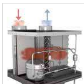
The air flows through the evaporator, giving up its heat energy.
