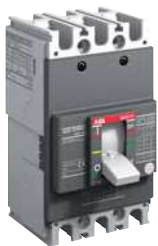
A1 100A TMF - Fixed (F) - 3 pole - Front terminals (F) - UL/CSA - Thermal-Magnetic (TMF) 240Vac
